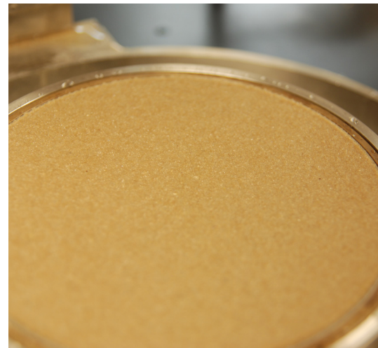
Pulp on handsheet mold
